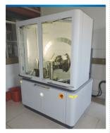
Empyrean, PANalytical–X-ray diffractometer equipped with a robotic arm sample exchanger. This is a high definition crystal analysing system with ultimate X-ray platform for the analysis of powders, thin films, nanomaterials and solid objects for industrial applications such as soil mineral analysis, cement industry, mines, metal manufacturers and crystal synthesis.
