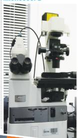
The MA200 inverted light microscope offers high stability, ease-of-use, with a large sample size option selection with both transmitted and reflected light modes which offers BF, DF, DIC, PH and limited florescence with high resolution lenses.
