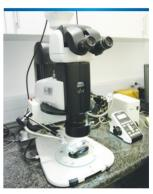
The Nikon SMZ25 stereomicroscope combines macro and micro imaging in one instrument for convenient viewing and manipulation of single cells to whole organisms.
