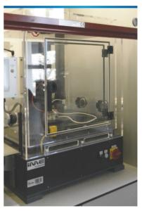
The EC-CLI is a unique electrospinning equipment with climate-control capabilities designed for demanding applications in which process control and reproducibility are crucial. Cylindrical collectors allow the fabrication of tubular nanofiber structures for tissue engineering.
