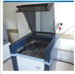
The S8 TIGER spectrometer is a high end XRF instrument that is used for elemental analysis in various industrial applications, including oil, lubricants, refinery, cement and mining samples. It is a highly automated and heavy duty system to handle a large number of samples.
